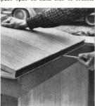
Use piano hinges for lids that open on top and for doors in front. Contact-cement sheet aluminum to lid bottoms; they'll be easy to wipe off
