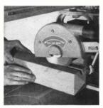
For lamp on corner post, run sheathed wire in trench from house connection up post in groove you can cut or have the lumber dealer do for you
